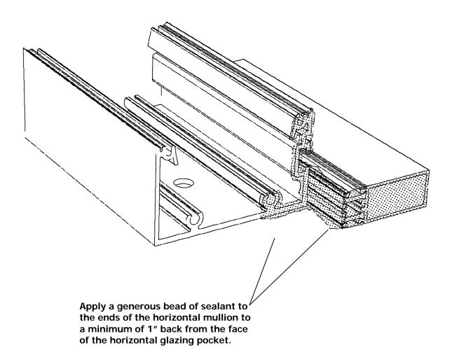
SSG HEAD & SILL HORIZONTALS WITH REVEAL AT SSG REVEAL JAMBS
