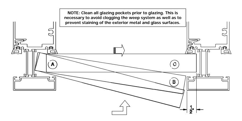
NOTE: The typical glass bite for the captured system is ½".
