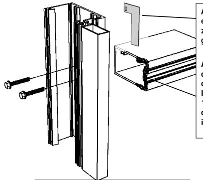
Apply H10Z Gasket to each end of the Horizontal. Trim excess gasket after assembly.
