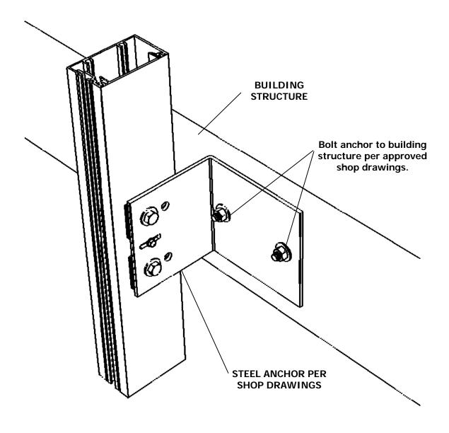
NOTE: The elevation of the structure must be within the adjustment limits of the anchoring system. See approved shop drawings for limitations.
