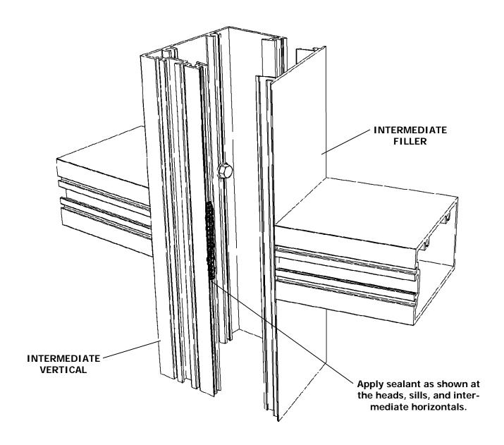
Note: Care should be taken when handling the frames to avoid damaging the edges of the fillers. A block of wood and "C" clamps should be used to aid in snapping the filler to the mullions.
