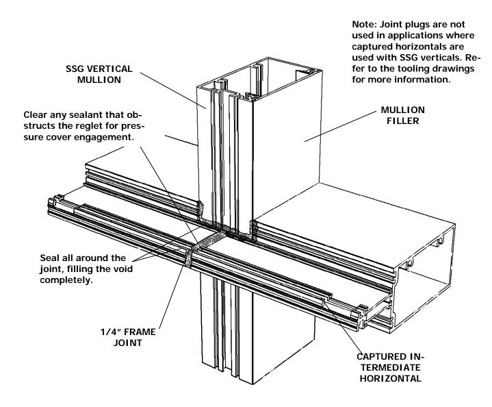
CAPTURED INTERMEDIATE HORIZONTAL AT SSG VERTICAL INTERSECTION
