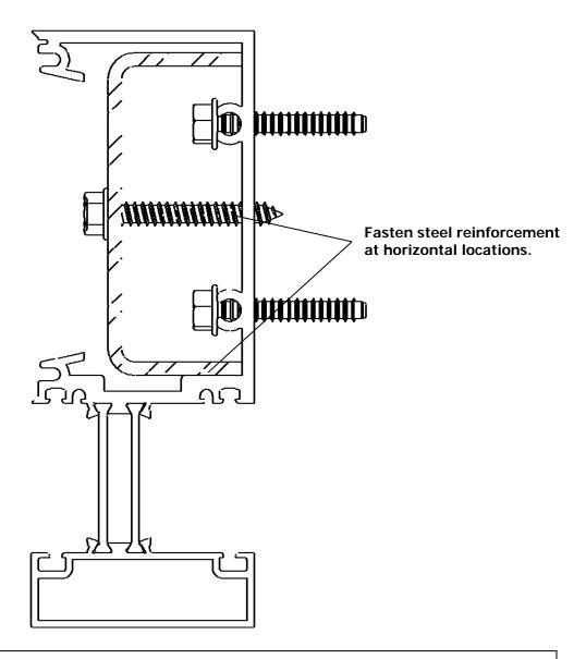
When steel reinforcement is factory installed into the mullions, fasteners will be used to prevent damage or slippage of the steel during shipment. This practice is also recommended for the customer on stock length orders.
