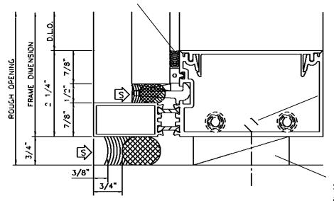
Anchor bolts (type and quantity as required by condition and loads. See Shop Drawings)
