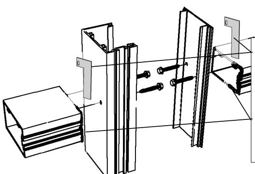
Apply H10Z Gasket to each end of the Horizontal. Trim excess gasket after assembly.
