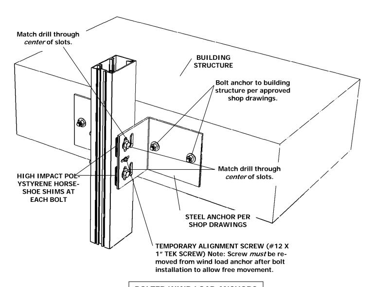
**BOLTED WIND LOAD ANCHORS**
