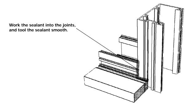
SSG SILL HORIZONTALS WITH REVEAL AT SSG VERTICAL MULLIONS (HEAD SIMILAR)
